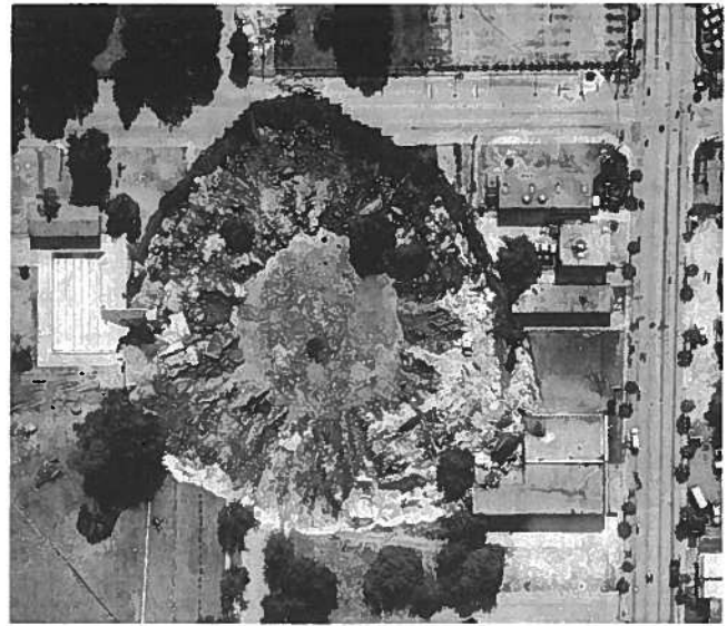
Fig. 8 — Overburden subsidence sinkhole, Winter Park.
